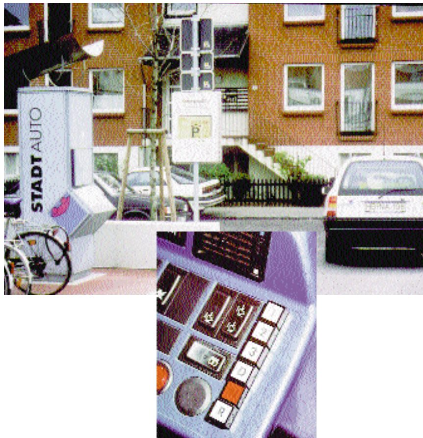
TOP: CAR SHARING STATION IN BREMEN. BOTTOM: CAR SHARE PANEL INSIDE OF CAR. THE USER IDENTIFIES HIMSELF WITH HIS PIN-CODE (MANUAL AT THE DASHBOARD). IF PIN IS RIGHT THAN THE IMMOBILISER IS RELEASED.
